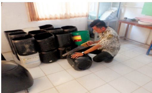
Figure 6.3 Process Of Making Garbage Bin From Used Plastic Jerry Can
