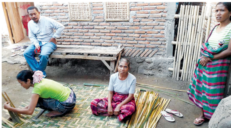
Figure 4.11 The Making of "Bedek" – Plaited Bamboo For House Wall
