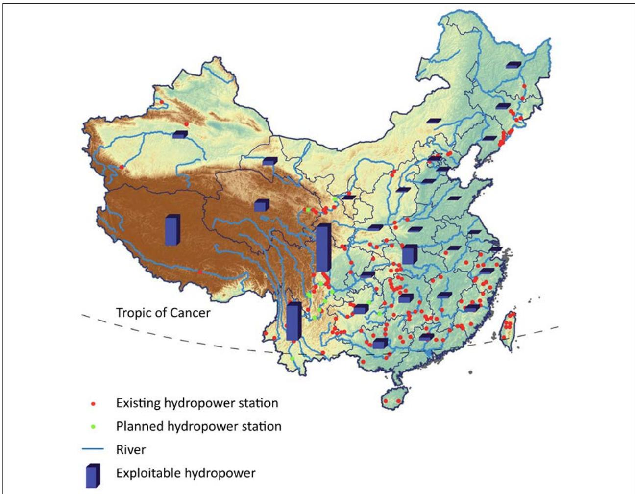
Figure 13: Distribution of hydropower resources and the major hydroelectric dams in China's mainland (2013 data). Blue blocks indicate the exploitable hydropower in the corresponding province. Tibet, Sichuan, and Yunnan host over two-thirds of total hydroelectric resources (Hu et al., 2013).
