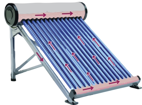
Figure 26: Rooftop Solar Collector.
