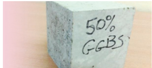
Figure 35: A Concrete Cube with 50% GGBS Content.
