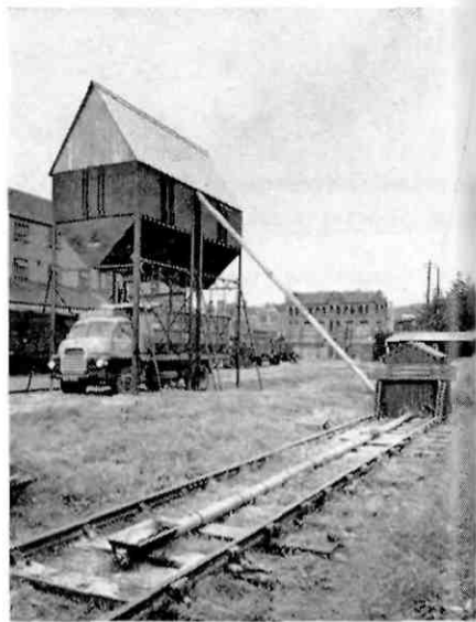
The mechanized handling of grain at this British milling company means that now one man does in less than an hour what it formerly took three men to do in twice the time. Manhandling is rare nowadays (Photo reproduced by courtesy of Messrs. A. and W. Evans, millers, Leicester)
