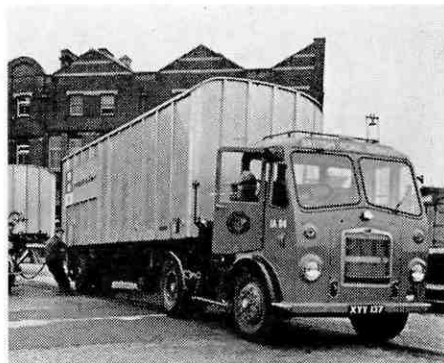
British Railways' new road-rail vehicle, the 'roadrailer' is lowered onto the rails. This vehicle combines the flexibility and convenience of road movement for collection and delivery of freight with the speed and economy of railways for the trunk haul (Photograph by British Railways)
