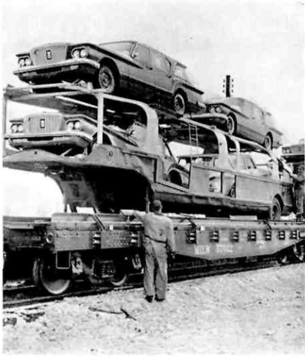
Four cars to a road trailer and two trailers to a railroad flatcar. This quick method of transportation (the 'piggyback') where goods are carried in wheeled vehicles – themselves used to bring them to the railhead and carry them forward from the rail terminal – is being increasingly exploited today, particularly in the United States
