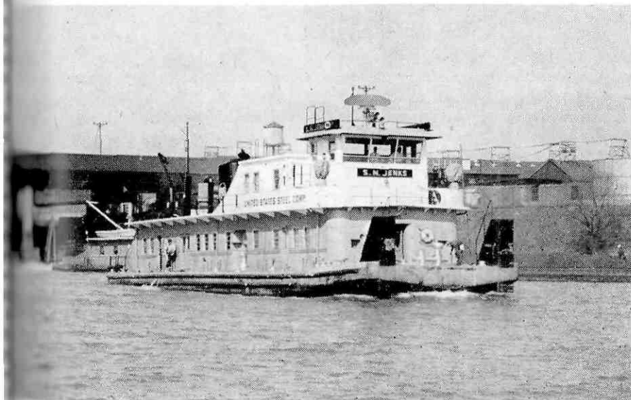
With its stainless steel hull and built-in air-conditioning unit, this vessel represents just about the latest development in river craft. Vessels of this type are now appearing in increasing numbers
