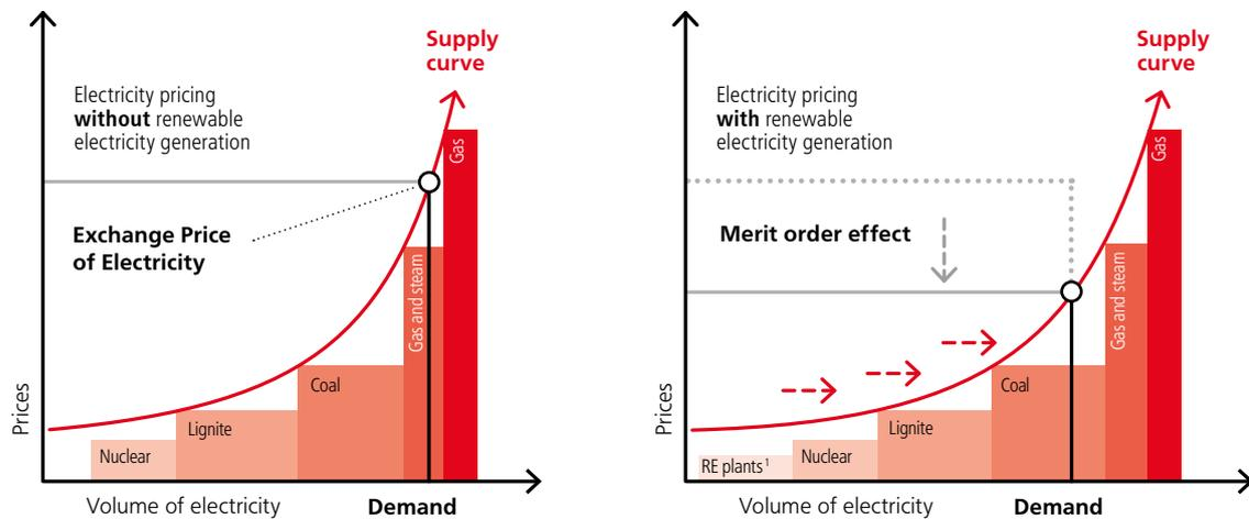
Note: owing to renewable energy plants, the supply curve shifts to the right in the right-hand figure. If demand is constant, this leads to a lower exchange price for electricity. The price difference corresponds to the merit order effect
