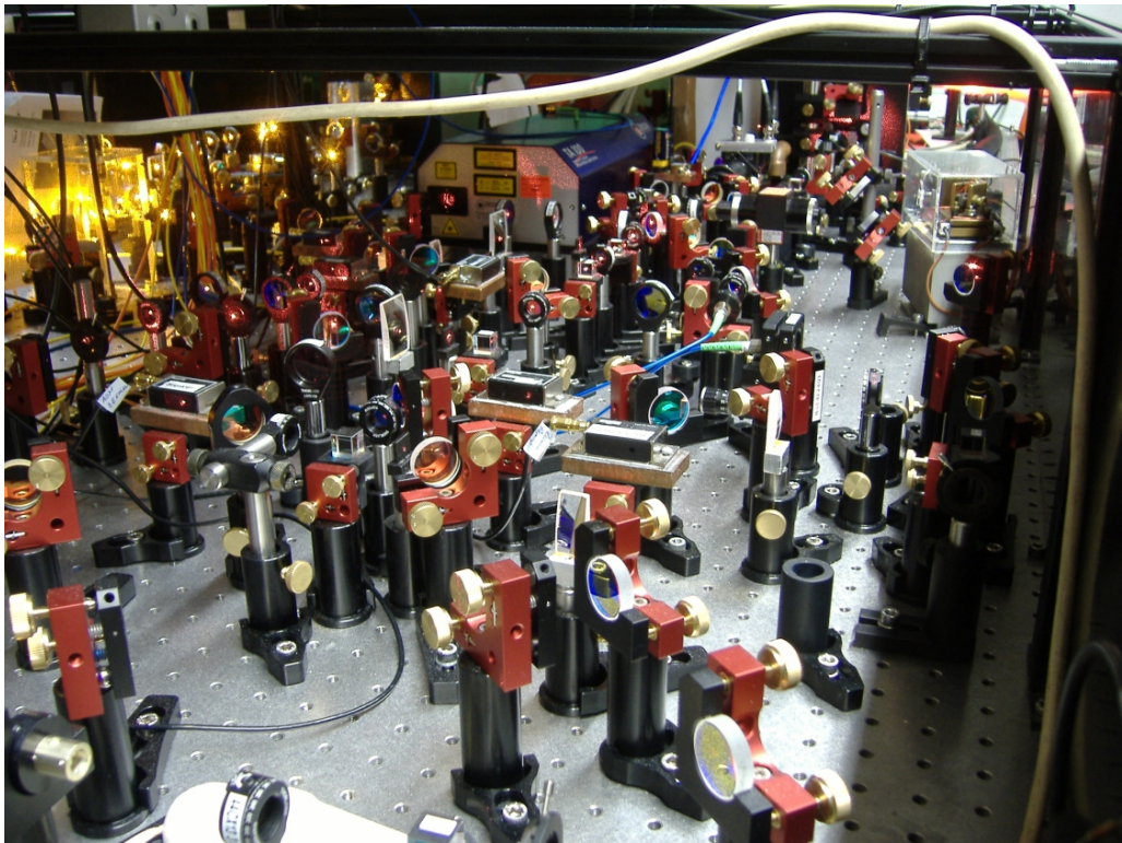
Figure 4.1: Optics of the laser system for lithium.
