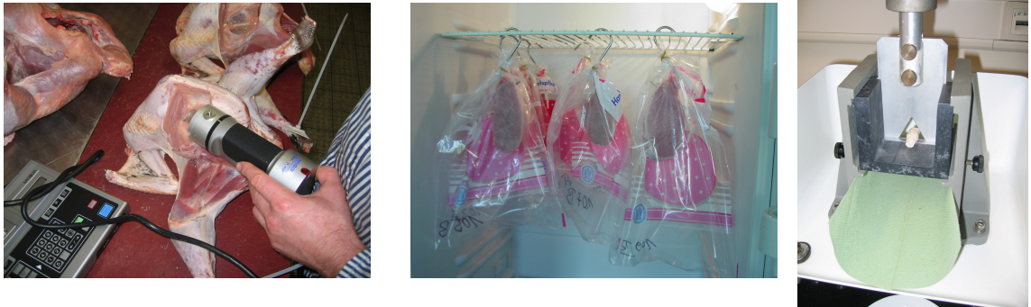
Figure 3: Minolta colour measurement (left), bag method (middle) and Instron (right)
