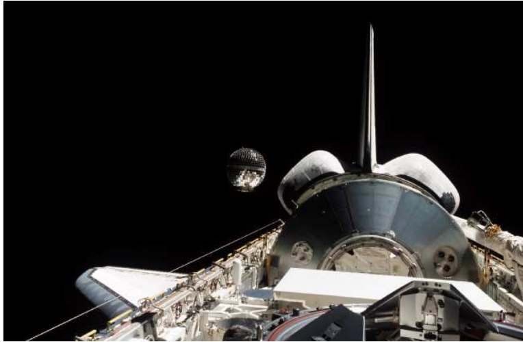
Figure 7.20: The STARSHINE1 satellite is released from the payload bay of a Space Shuttle Orbiter. (Taken from [26])
