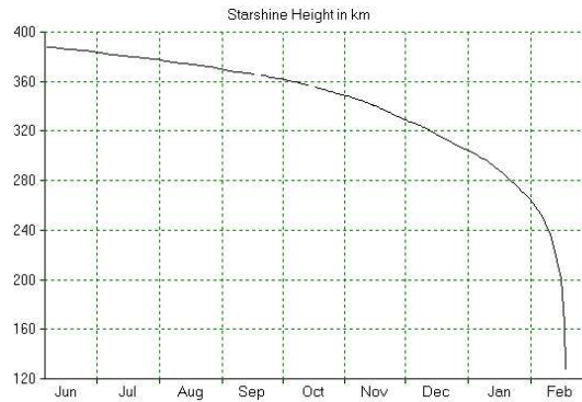
Figure 7.22: STARSHINE1 orbit decay as computed from flight data analysis [9]. The entry interface at 120 km is reached after approximately 259 days.
