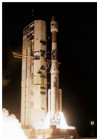
Figure 7.50: An Ariane 44LP lifting off from a launch pad in French Guiana. The solid and liquid boosters attached to the main body are clearly visible. (Courtesy of ESA)
