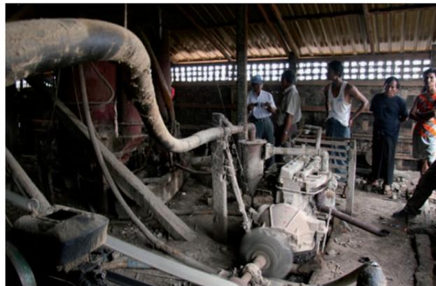
Abbildung 9: Biomasse-Vergaser in Myanmar
