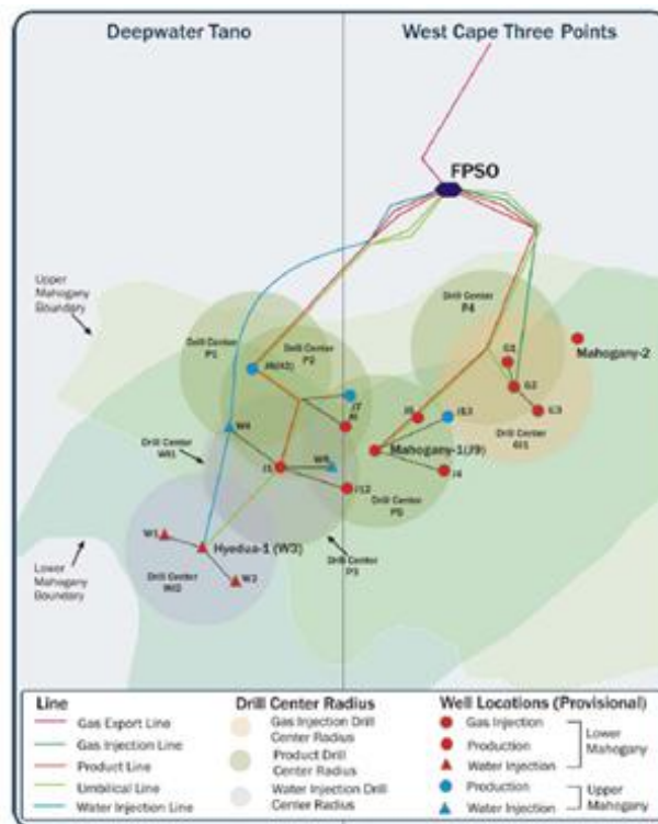
Image 2: Drill Centre Locations and Associated Flowlines, Injection Lines and Umbilicals. [Tullow Oil, 2009]
