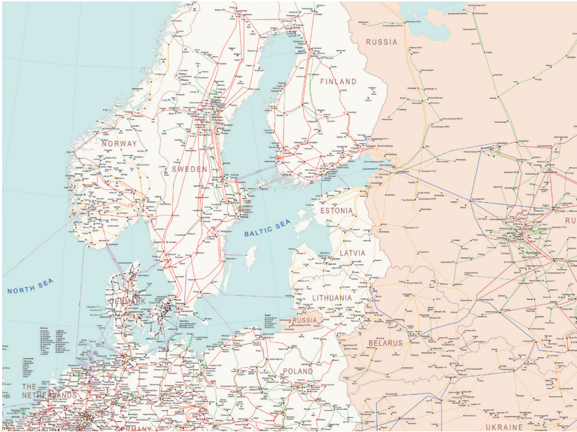
Picture 1. Electricity transmission system in the Baltic Sea Region
