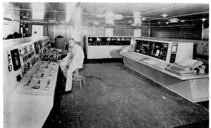
Above: The system of automated engine room control installed on the Dolabella enables an oil tanker to be 'driven' in normal circumstances by one man from the bridge, with the engine room unattended. Below: The cargo control room. Loading and discharging operations can be controlled by one man. (Photos: Shell)
