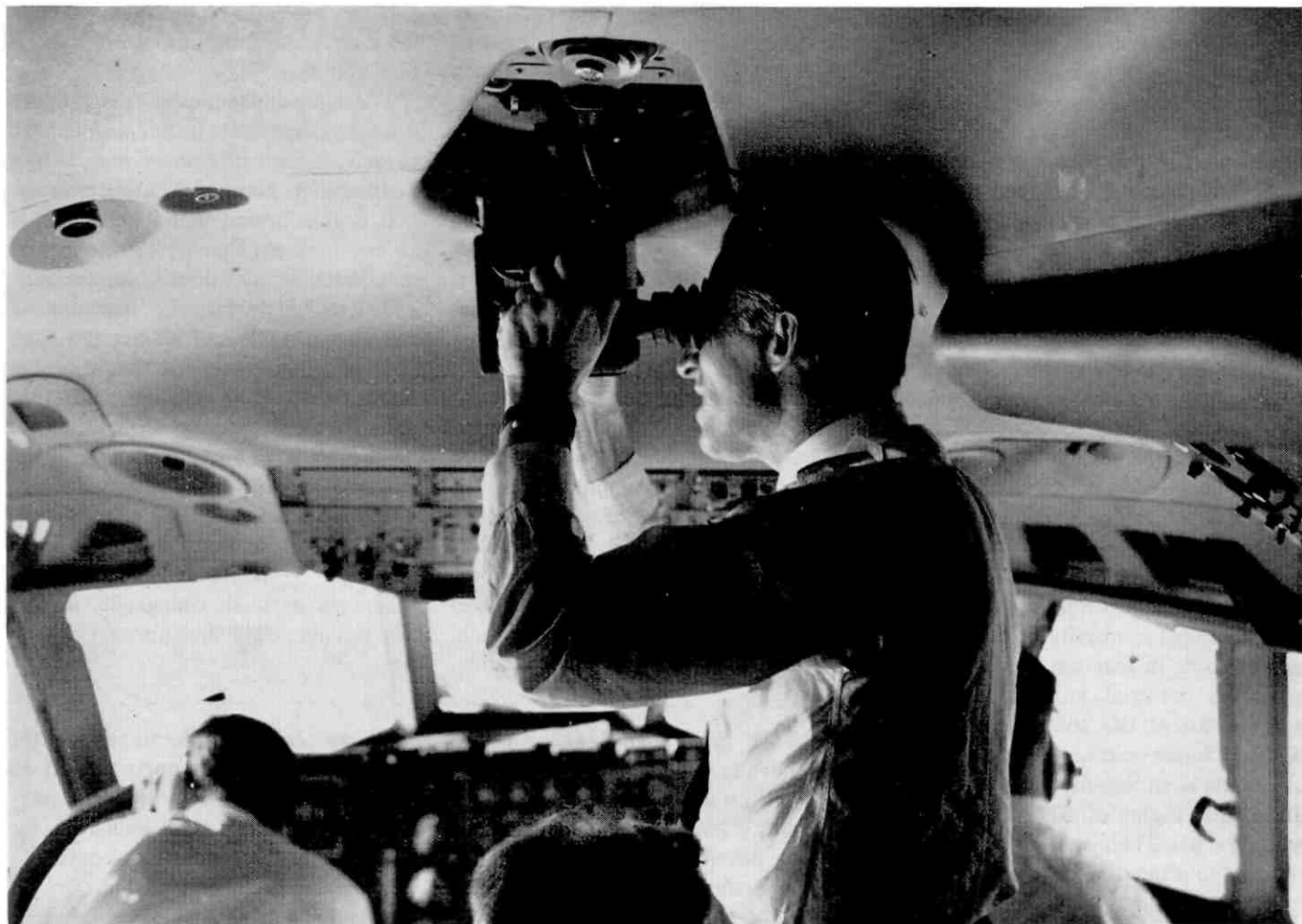
Navigating officer aboard a British Overseas Airways Corporation VC10 using the periscopic sextant during flight.
