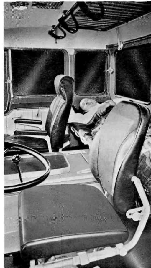
Bunks in the driver's cab are recommended for short rests rather than for overnight sleeping accommodation.
