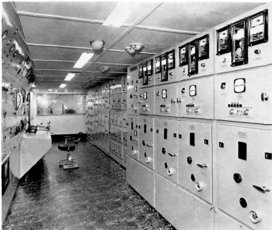
The control room of the British motor vessel, Clan Ramsay. This refrigerated cargo vessel, launched in 1964, has been equipped with centralized control of all its running machinery.
