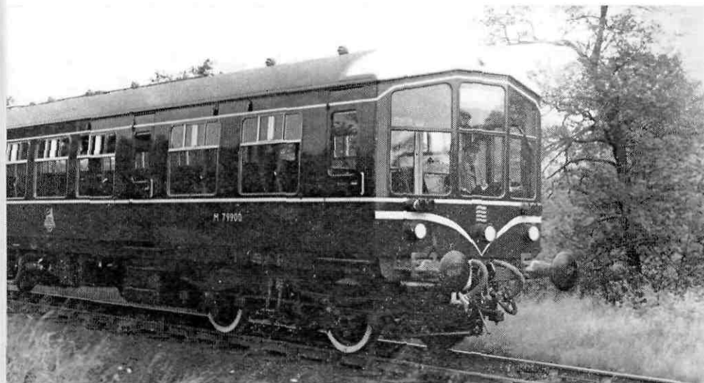
British Railways diesel railcar designed to be used in subsidiary branch line services.
