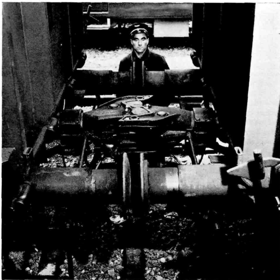
A very high proportion of accidents to railway personnel occur to employees engaged in coupling operations. An efficient automatic coupling system would remove the need for railwaymen to step between wagons for any part of the coupling operation.
