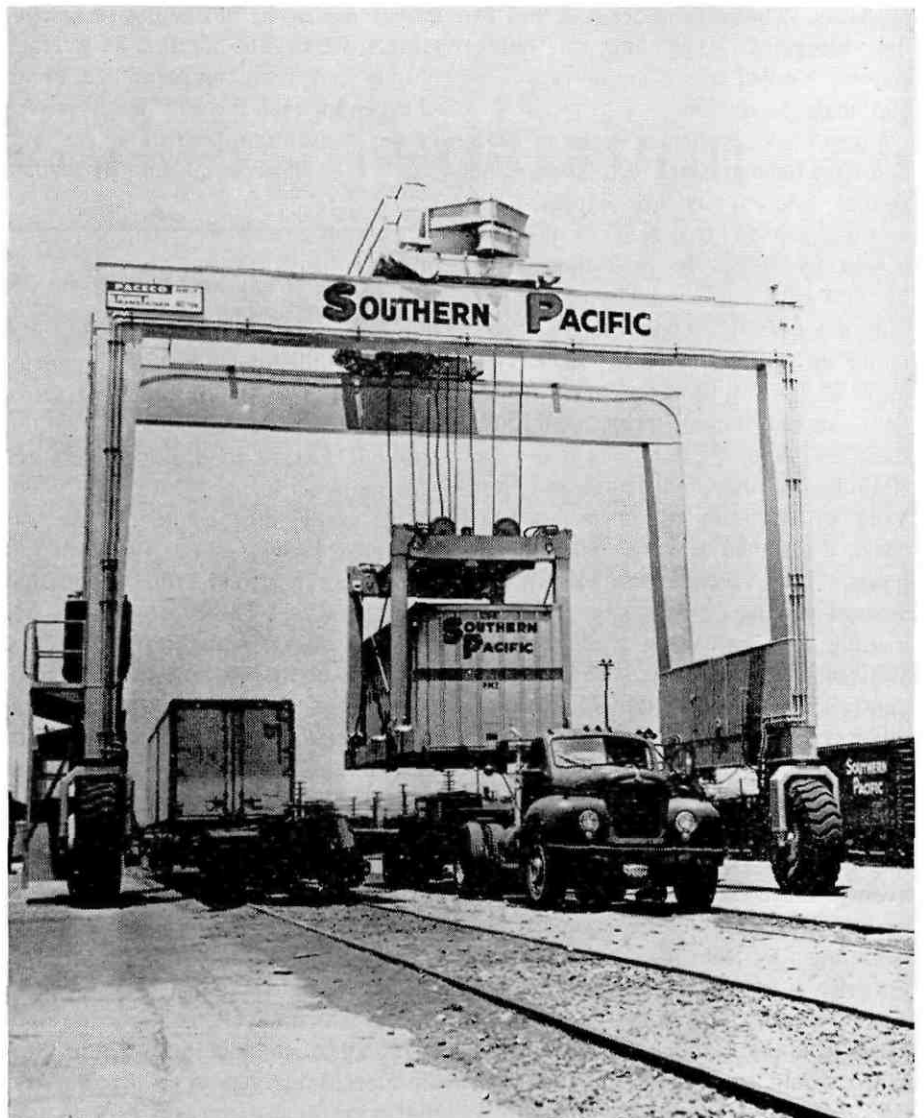
Mobile gantry crane can lift trucks, vans and trailers on and off flatcars in three minutes. Piggyback operation is growing rapidly in America (USIS photo)
