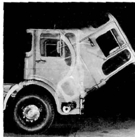
The new 'ergomatic' tilting cab is an all steel structure. The lower frontal assembly incorporates reinforced members to give good protection to the driver in an accident
