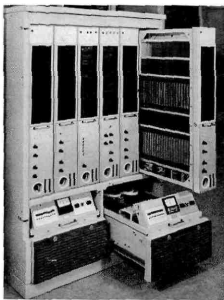
SATCO computer cabinet – memory rack and power supply unit pulled out – (Photo NV Hollandse Signaal Apparaten)
