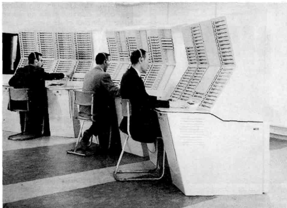
Automatic airways flight progress boards. This photograph was taken during training of air traffic control personnel at Schiphol Airport (Photo NV Hollandse Signaal Apparaten)
