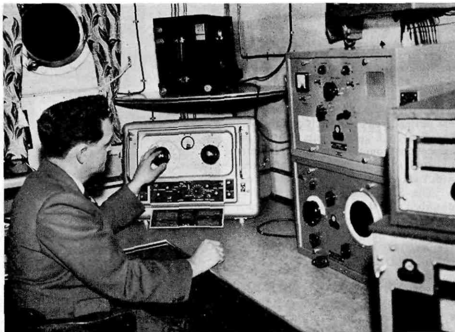
Marconi Marine equipment in radio room of the trawler 'Stella Leonis' includes automatic direction-finder, which is being tuned by the radio operator (Marconi Marine photograph)
