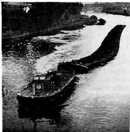
A train of special compartment boats carrying coal on the Aire and Calder Navigation
