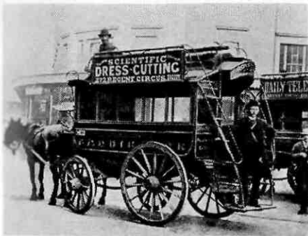
A London omnibus of 1887 outside London Bridge station. The upper deck has a 'knife-board' seat — two benches divided by a common back rest running lengthwise down the carriage. The outside staircase was a relatively late innovation; at first passengers had to clamber up however they could
