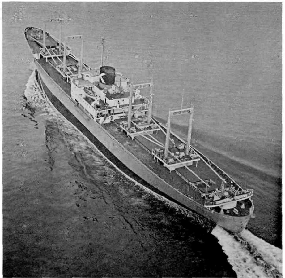
The Japanese cargo liner, MISSISSIPPI MARU, is claimed to incorporate the world's most advanced automation systems. This 12,000 dwt ship can operate with a crew of 28
