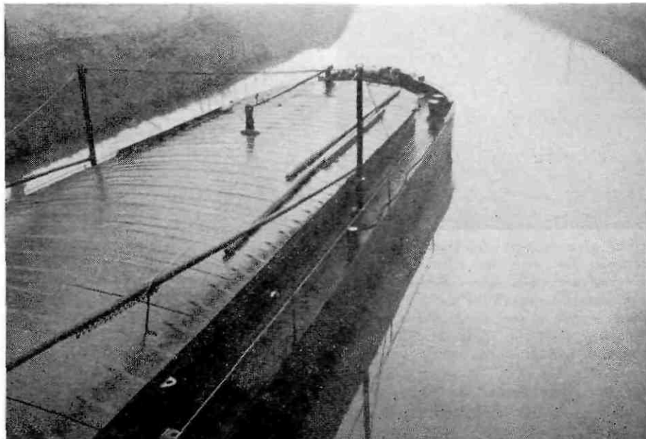
Barge equipped with a guard rail. Falling overboard is one of the most frequent accidents experienced in inland navigation, and the risk of this happening can very easily be minimised by fitting a simple rail such as this for the convenience of members of the boat's crew
