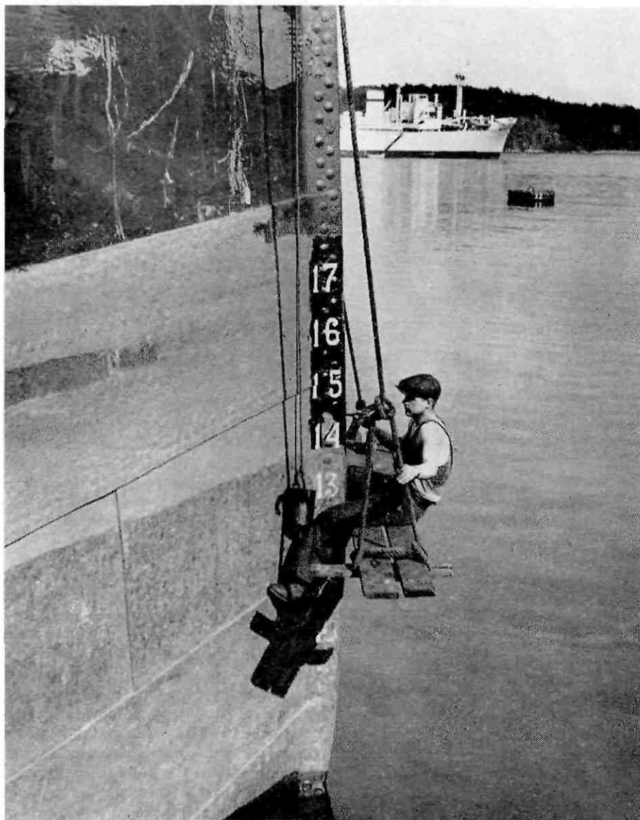
An important part of security of employment for seafarers is protection at work. The man in the picture should be provided with a lifeline for the sort of work he is doing
