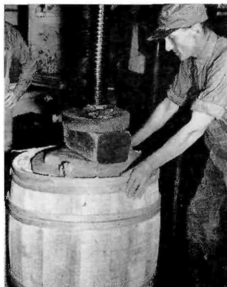
Cod is caught in the inshore waters and on the deep-sea banks off Canada's Atlantic coast, and a large proportion of the catch is salted and dried for marketing. This power press in Lunenburg, Nova Scotia, packs 500 lbs of cod into barrels
