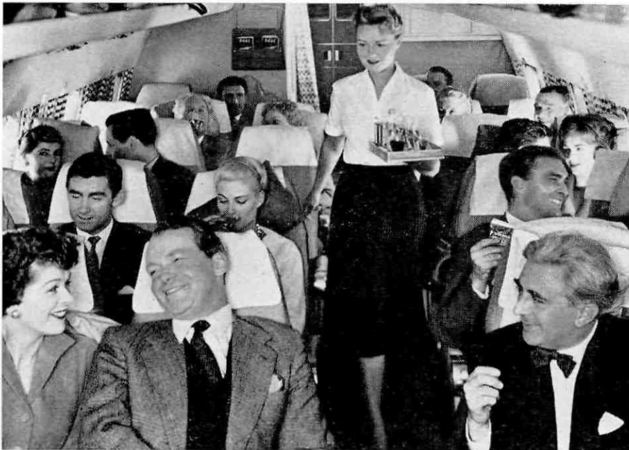
For efficient, safe and comfortable working conditions the fore and aft aisle should have a minimum width of 24 inches (BOAC photograph)
