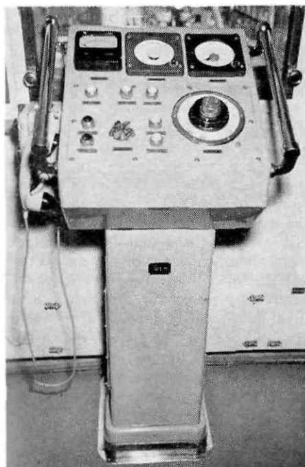
The 'Kinkasan Maru' is the first cargo liner in the world to have a main engine remote-control console in the wheelhouse of the bridge (shown in this photograph). American shipowners are beginning to introduce more widespread automation, and an inquiry is being held into the effects this will have on employment in the industry (Photo lent by 'Shipbuilding and Shipping Record')
