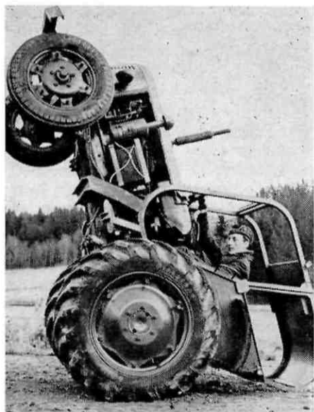
The back of this new tractor cab developed in Sweden is built so that, if the tractor rears up, it cannot capsize completely. In tests where the tractor has been overturned sideways or backwards, the steel structure has afforded the driver maximum protection
