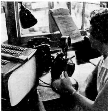
At Kings Cross and Paddington stations, London, current passenger train information is transmitted from the signal box by means of closed circuit television and simultaneously displayed in the various offices requiring it
