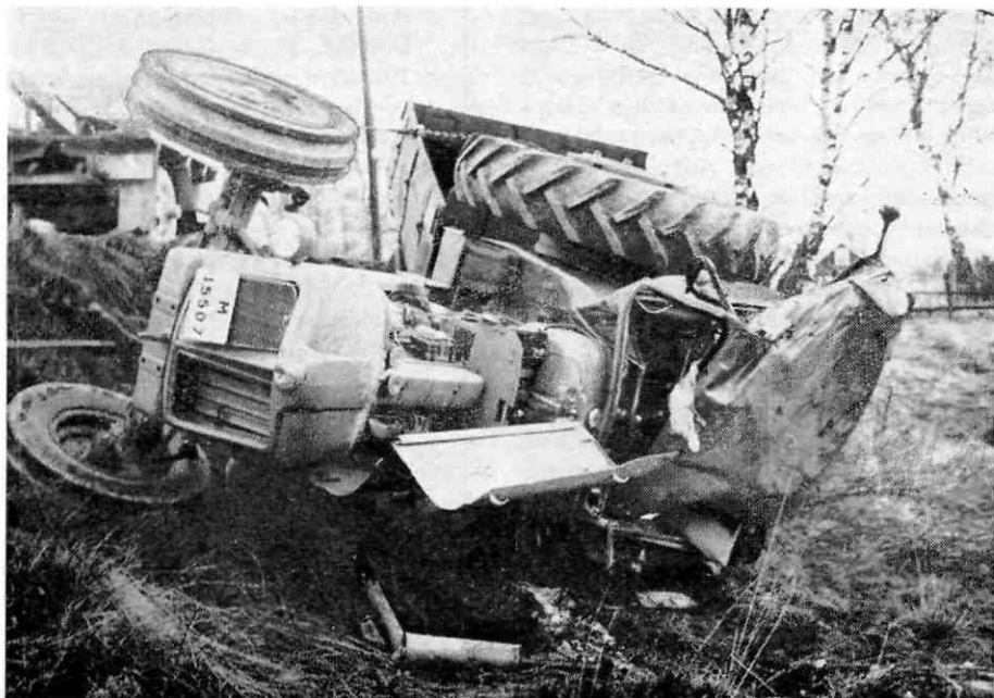
The tractor is a dangerous vehicle — not because of its speed, but because of its particular design and construction. Owing to the uneven distribution of its weight it tips over easily or rears up like a horse. In these cases the driver can be seriously, if not fatally, injured
