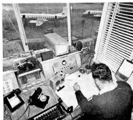
In order to maintain efficiency and ensure safety, the highest standards of vigilance and professional competence are indispensable in flying. These standards apply also to the ground control staff. It is expedient that they should have at their disposal all the aids which modern technology can offer. This picture shows the closed circuit television in use at London (Heathrow) Airport in air traffic control operations
