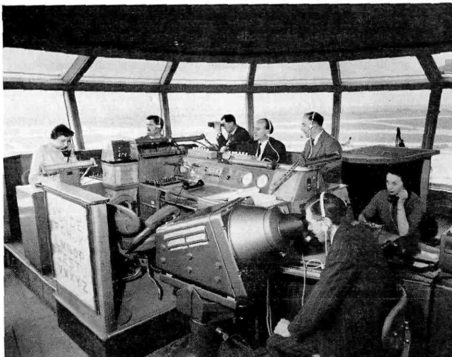
The Air Traffic Control Officer has as his primary aids Radio Telephony (R/T) in the Very High Frequency Band, and Radar. The former enables him to talk directly to the pilot of the aircraft over fairly long distances, the latter permits constant surveillance of the airspace to ensure that separation standards between aircraft are not in any way infringed
