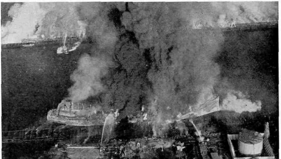
One of the photos from 'Fire Aboard' showing the 10,342-ton tanker 'Markay' on fire in Los Angeles Harbour. Note the fires on both sides of the 600-ft.-wide slip. The tanker was loading butane at the time of the explosion which led to this disastrous outbreak of fire
