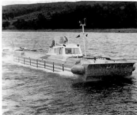
Bow-end view of the experimental sidewall hovercraft which will probably be utilized as a passenger-carrying ferry in Britain during the course of next year. The craft will carry between fifty and seventy passengers and will have a maximum speed of 35 knots. (Photo courtesy P.A.-Reuter)
