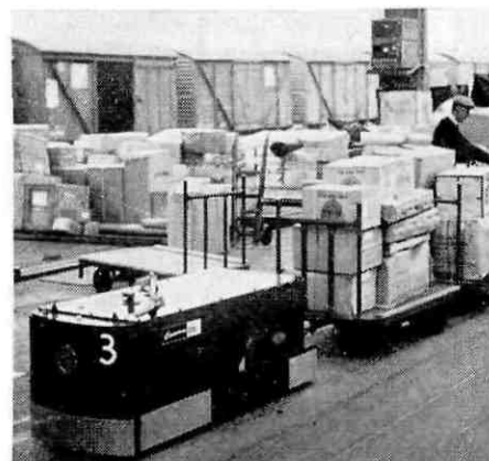
Loading a trailer with parcels at Wolverhampton. One of the Robotugs can be seen in close-up in the foreground. Aim of the scheme, says British Railways, is greater efficiency to enable the movement of a larger tonnage with considerably less manual effort
