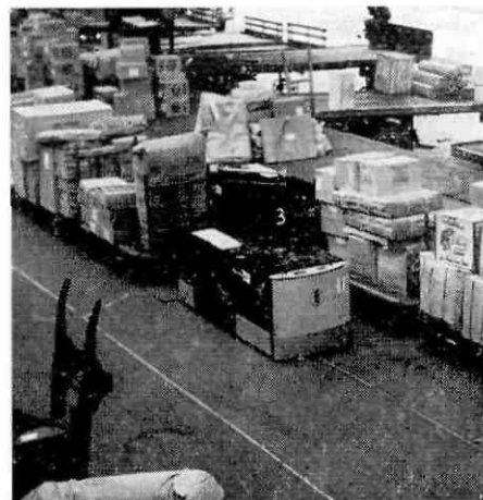
Two Robotug driverless trucks, hauling trains of trailers, pass each other on the platform of Wolverhampton's Herbert Street Goods Station, where five Robotugs have recently been installed for inwards goods handling
