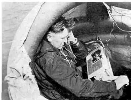
Strapped to the knees of the operator, and powered by a handdriven generator, the Lifeline's transmitter/receiver can be used by unskilled personnel under difficult conditions. Transistors have been used to reduce bulk (Photo: Marconi Marine International)
