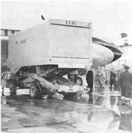
The Cargomaster, an aircraft loading machine recently put into service by BOAC, cuts loading time by some 25 per cent and unloading time by as much as 50 per cent. A number of these machines are to be used in connection with the all-cargo services operating across the Atlantic
