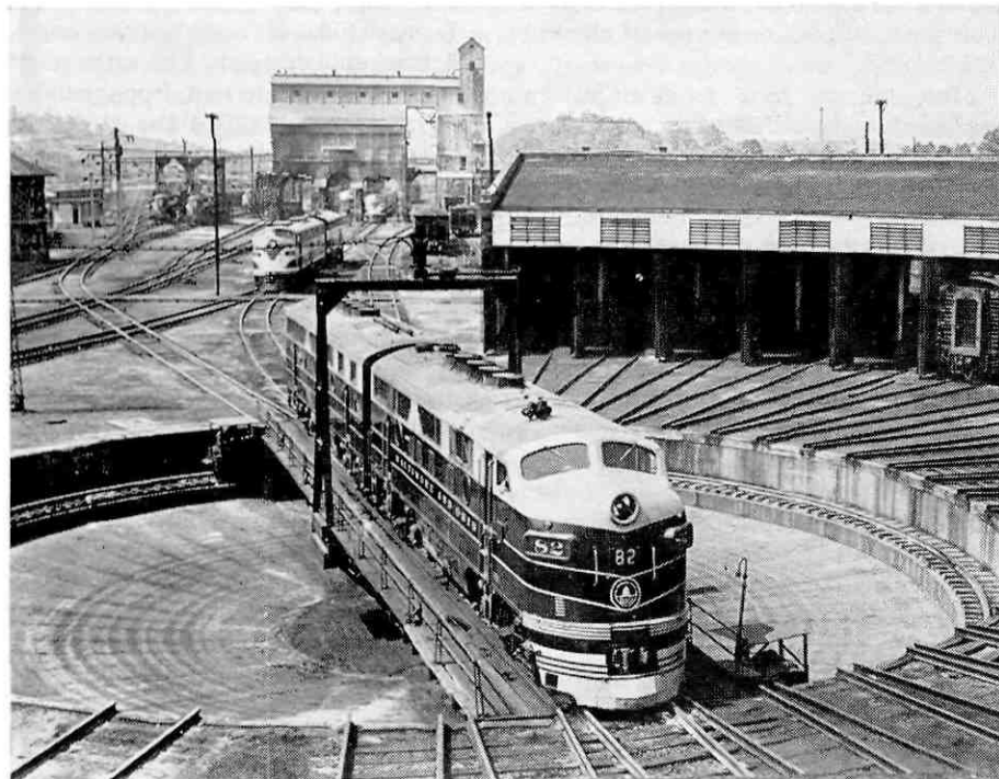
A modern United States diesel locomotive is lined up on the turntable with the track leading to its stall. In the yard, too, the US fireman-helper must be alert and keep a vigilant look-out for anything which might create an unforeseen hazard or an unsafe condition (An AAR photograph)
