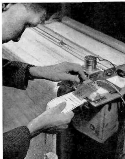
Sensing fingers read the information by making electrical contact through the many punch-holes
