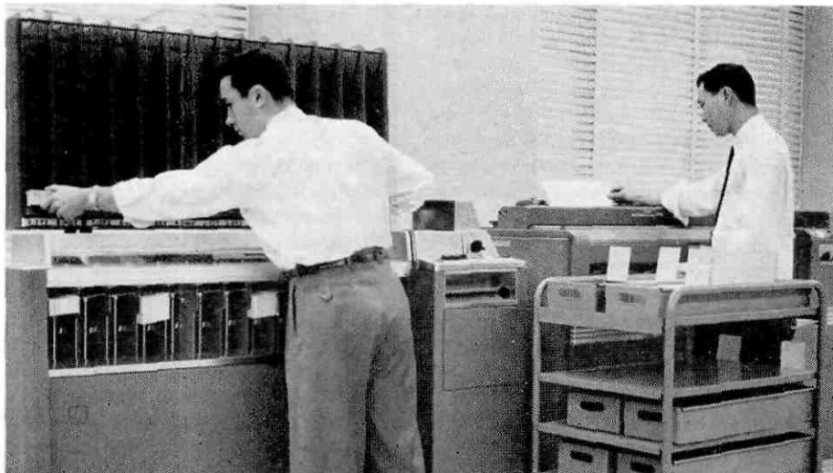
Jimmy Walker (left) is busy operating an electronic sorter that shuffles cards at really astonishing speeds to match punched holes, while his colleague is engaged in looking after a statistical sorter
