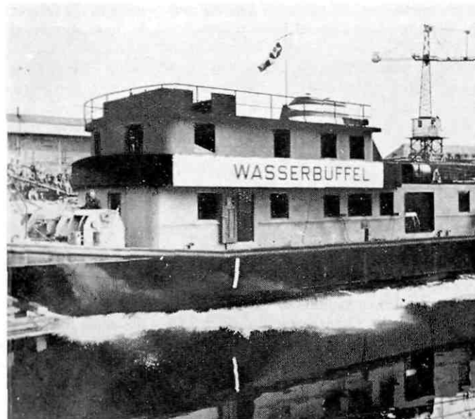
One of the most recent developments on West European waterways is the introduction of push propulsion, a system which has for long been successfully used in the United States. As shown here, a pushboat like the 'Wasserbüffel' is capable of pushing anything from four to six crewless barges
