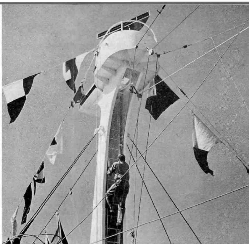
From the top of a mast – in the photo here the mast of a super-tanker – this radar antenna scans a wide area with unflinching vigilance. This antenna is set eighty feet high
