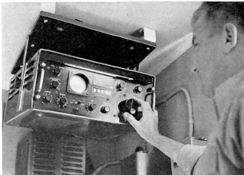
The new electronic device 'loran' (the name is taken from 'long range navigation') times signals from two pairs of special transmitters. Unaffected by atmospheric tricks, it plots results with pin-point accuracy — a far cry from the methods of old
