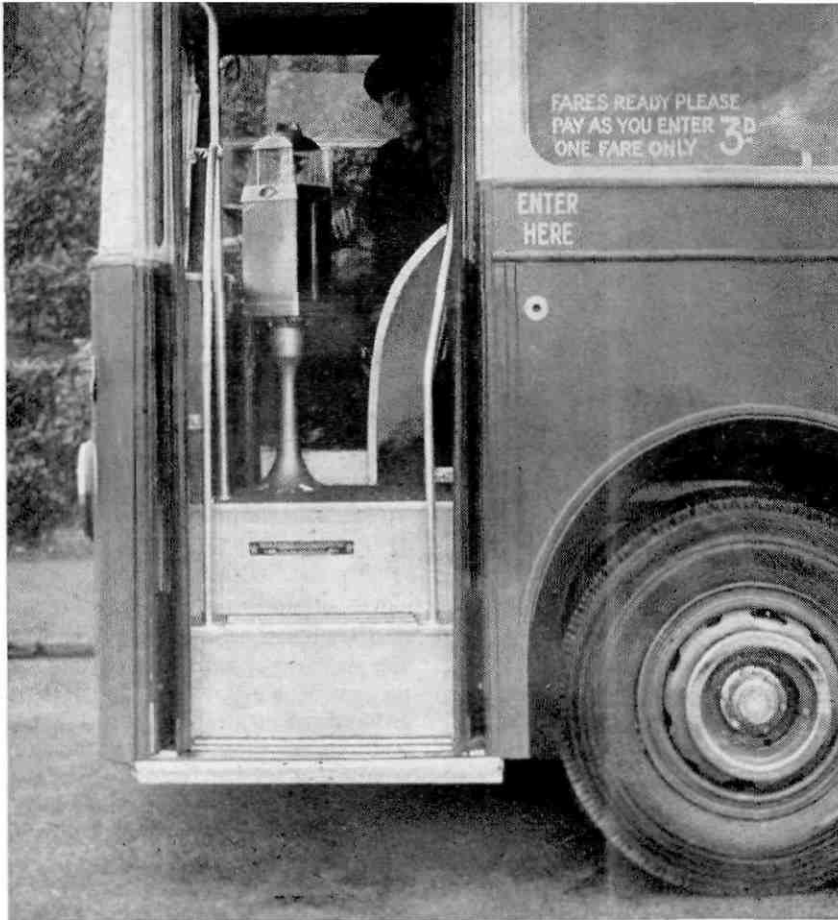
An experimental one-man bus built for use in Dundee, Scotland. It was designed on American lines and some modified American equipment was used. Passengers pay a flat-rate fare by inserting their coins in a meter; no tickets are issued at all (Photo reproduced by kind permission of 'Modern Transport')
