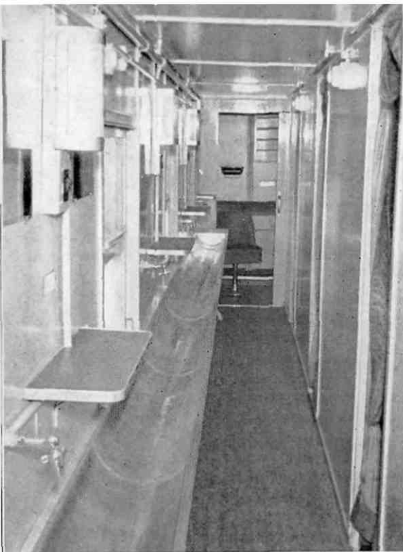
The German Federal Railways study the comfort of lorry drivers accompanying their vehicles being hauled by 'piggyback'. Washing and sleeping facilities are provided in a special car on the goods train. (Photo German Federal Railways)
