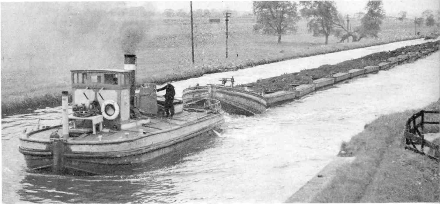
A compartment tug with a full train of nineteen compartment boats in tow carrying 760 tons of West Yorkshire coal to Goole for shipment. British Docks and Inland Waterways' Executive photo taken on a section of the Knottingley & Goole Canal
