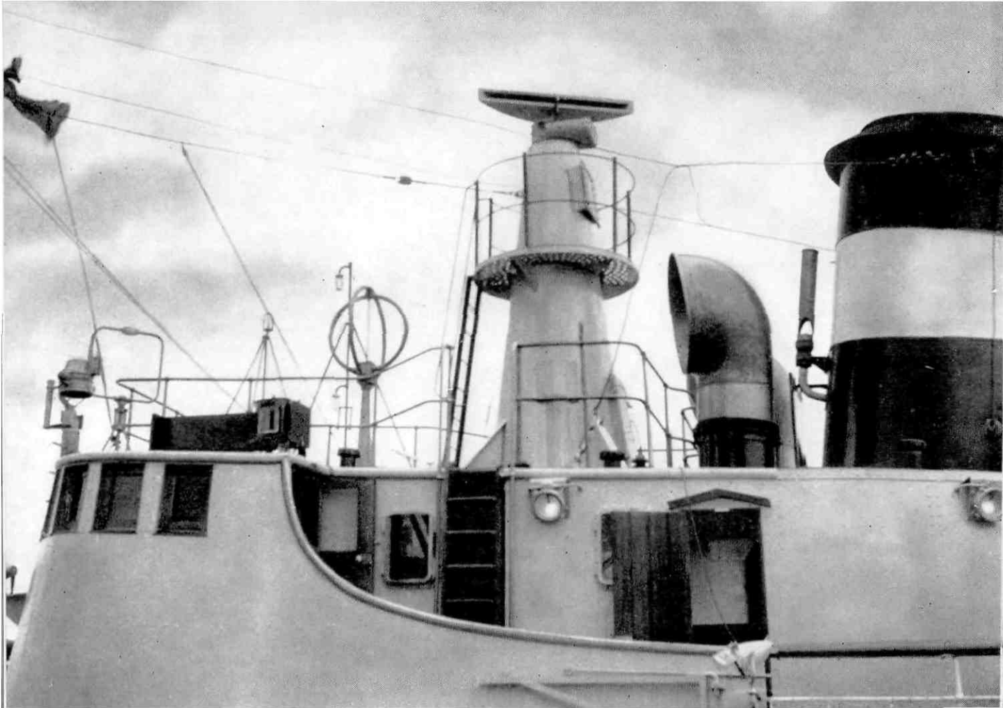
The scope of a modern trawler's radio aids to navigation, showing two direction-finder loop aerials and a radar scanner
