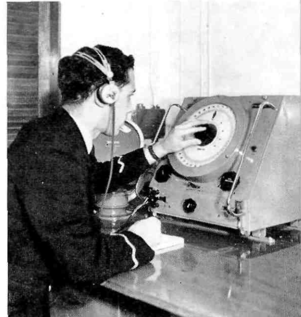
The radio officer of a liner taking a bearing on a shore radio beacon station by means of the 'Lodestone' direction-finder
