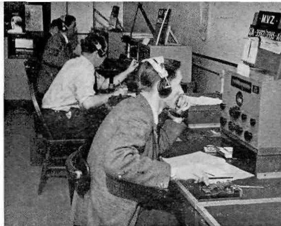
Behind the scenes in the radio section of a large modern airport. Both radio-telephony (centre) and wireless telegraphy are used to contact aircraft when in flight
