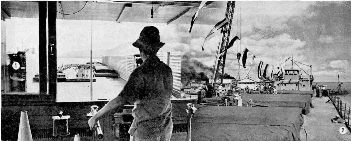
1) In the wheelhouse, a pilot manoeuvres a towboat through canal locks on the Ohio River. The towboat is capable of moving as many as 30 fully-loaded barges. 2) One of the many large self-propelled freight barges which ply along the Tennessee River
